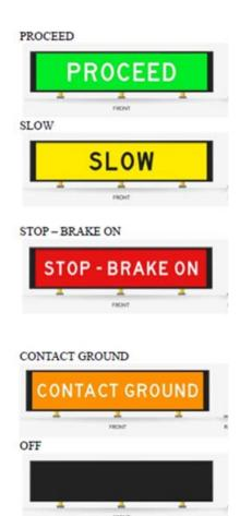
The variable message sign is a secondary means of communication controlled by the de-icing platform coordinator in support of the instructions communicated by VHF. VHF communication has priority over the indications as displayed on the variable message signs.
